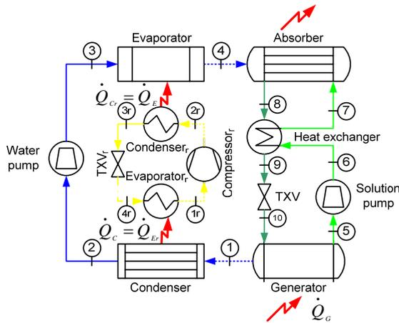
Figure 1. Diagram of the CAHT cycle.
