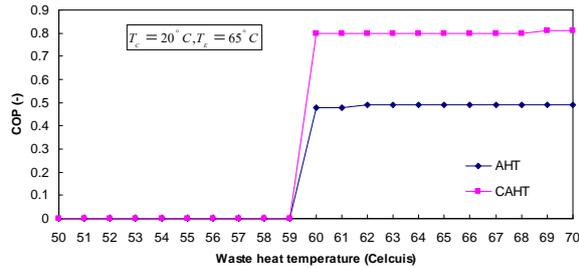
**Figure 4.** The overall COP of the normal AHT and the CAHT.
