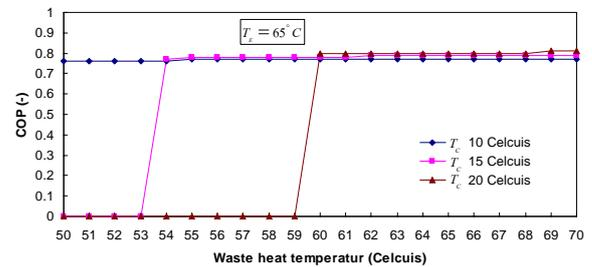
**Figure 2.** The effect of the AHT  $T_c$  on the overall COP.
